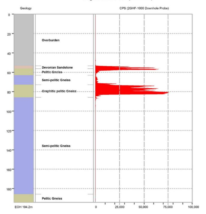
5) Here's the Gamma Log Profile for Fission #Uranium \$FCU's world-record drill hole PLS17-METC that contained a continuous 30-storey tall set of high-grade U core sections, 108m at Average Grade of 8.46% #U3O8. Best mineralized hole drilled worldwide for any mined metal in 2018
