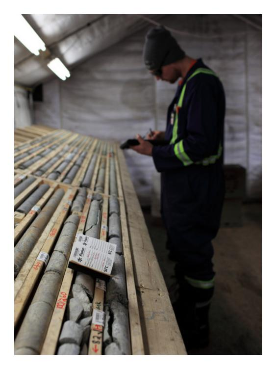
4) After an exploration hole has been drilled & all core samples recovered, an instrument called a Downhole Gamma Probe is lowered to the bottom & recovered, constantly measuring #uranium radioactivity in a 360 degree sweep to produce a complete Gamma Log Profile for each hole.
