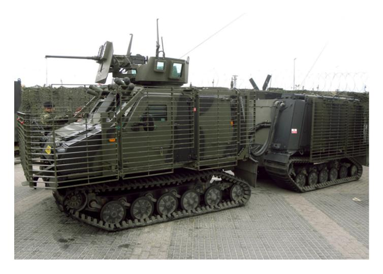
Having this low rear idler (typically somewhere between level with the other road wheels and marginally higher than to give a slight rear track angle of around 4°) means more ground contact area, more road wheels to bear the weight and so overall lower ground pressure
