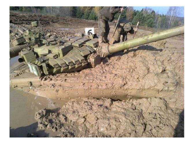
The issue is not just that the belly is taking loading that should be on the tracks to ensure they maintain grip on the terrain, it is also that any contact with the belly creates enormous levels of belly drag – a shear force frictional resistance to further movement
