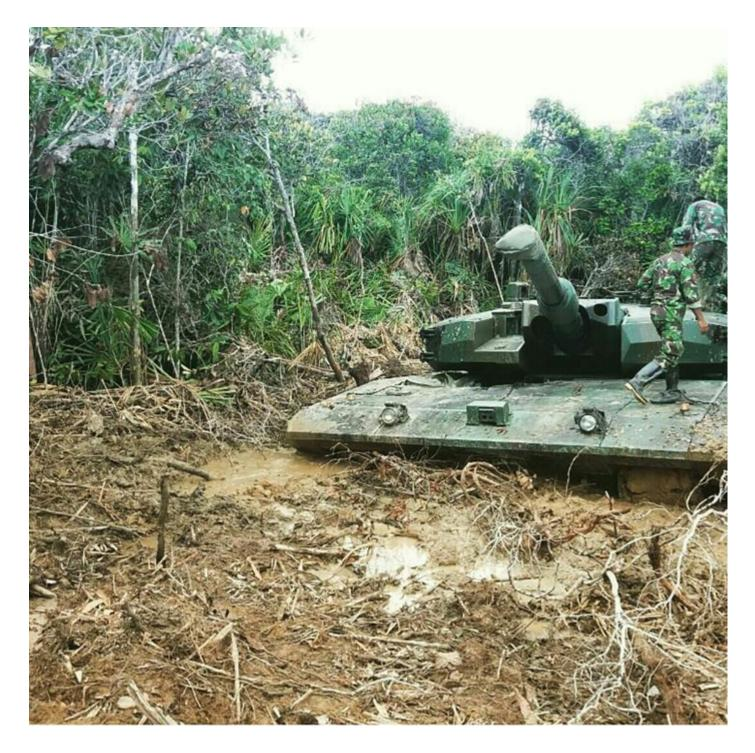
Belly loading is a cascade situation. With the belly only contacting terrain in a situation where mobility is already challenging and ground pressure/grip maybe be failing, contact of the belly begins to transfer load from tracks to hull, further reducing the tractive performance
