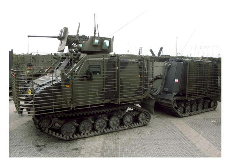
Having this low rear idler (typically somewhere between level with the other road wheels and marginally higher than to give a slight rear track angle of around 4°) means more ground contact area, more road wheels to bear the weight and so overall lower ground pressure
