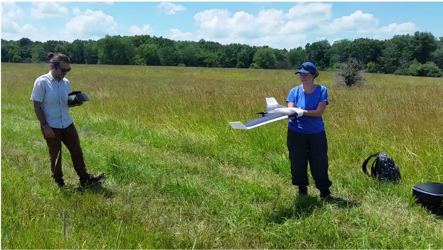
Ryan flew this puppy over all of Nachusa (how many flights, Ryan?), and we compared indices arrived f the sensor (e.g. NDVI and many others) to the plant/soil data we'd collected at the local scale.
