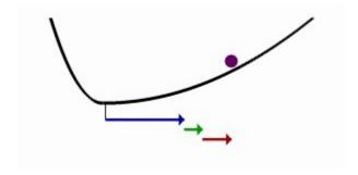
An electron (purple) is being pushed side-to-side by a sinusoidally-oscillating force, i.e. the light's electric field. But because the electron is in an anharmonic potential energy environment (black curve), the electron motion is not sinusoidal.
