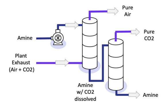
The amine selectively "dissolves" the CO2 in the first column, while letting the rest of the air pass through.
