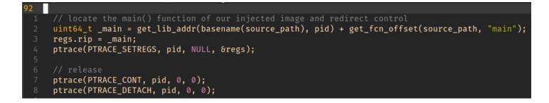
Finally we can detach the parent process.
