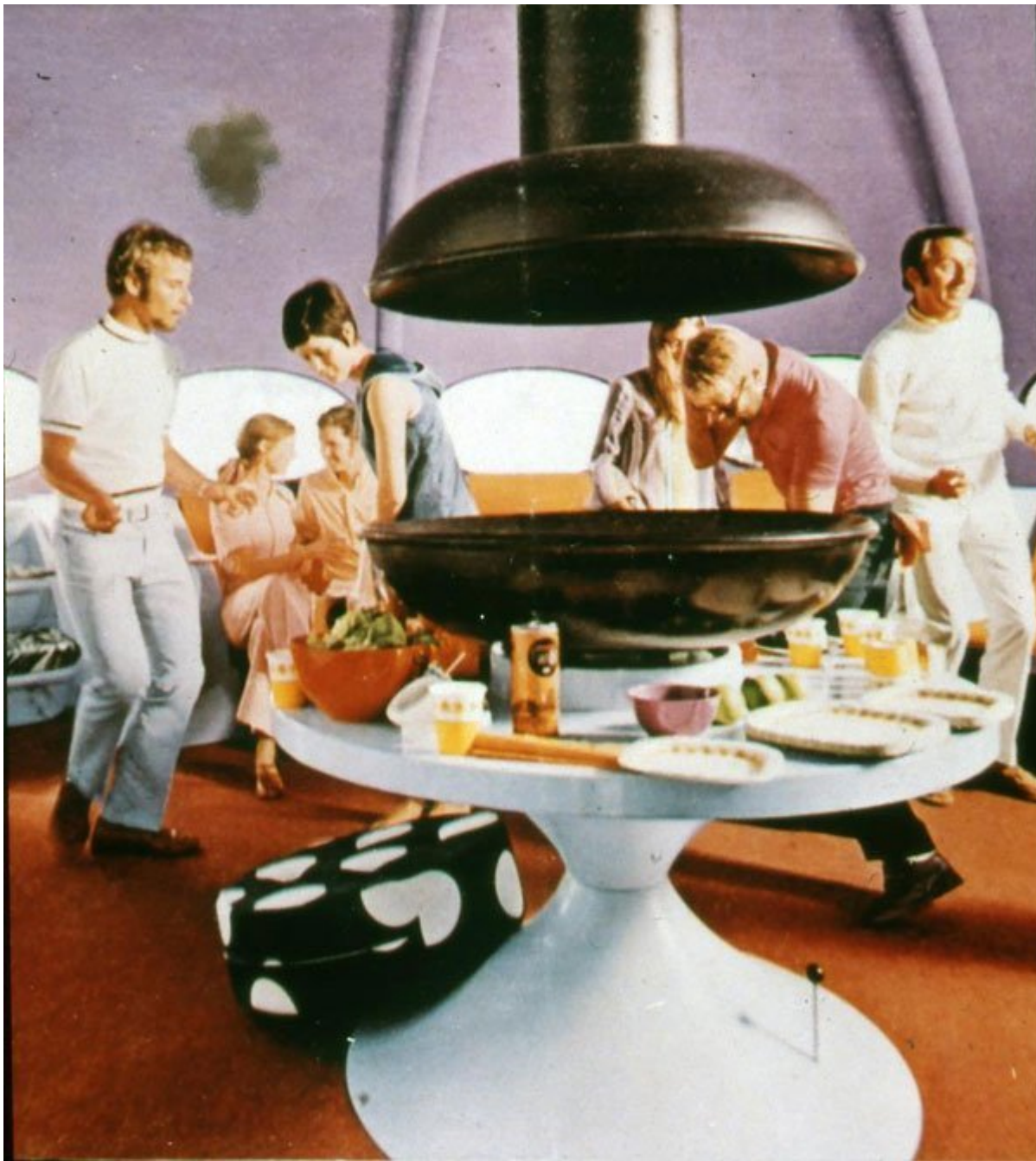
The Futuro was made of fibreglass- reinforced polyester and was light enough to be towed to any location. You literally moved house.
