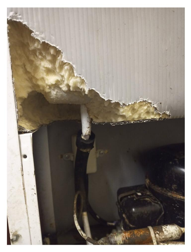
OK. Calm down. It's not the end of the world. I can repair it. Clean it. THOUROUGHLY. And plate the corner. Or, buy a new fridge...even though I can't really afford to ATM. So, calm down. Let's check they haven't punctured the suction line and
