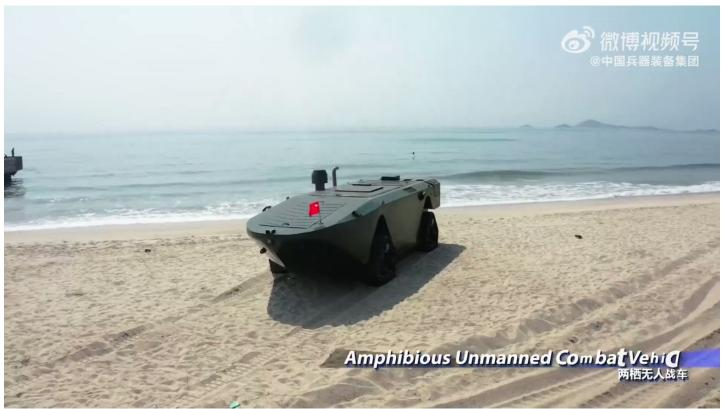
This particular UGV can retract its tracks, allowing it to travel on water like a speedboat
