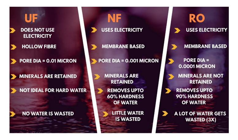
UF is much cheaper but its downside is that it can't be used for very hard water.
