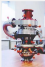
Cryogenic Engine - Turbo Pump, Injector Head, Gas Generator, Booster Pumps, Interfaces And Start Up Systems
