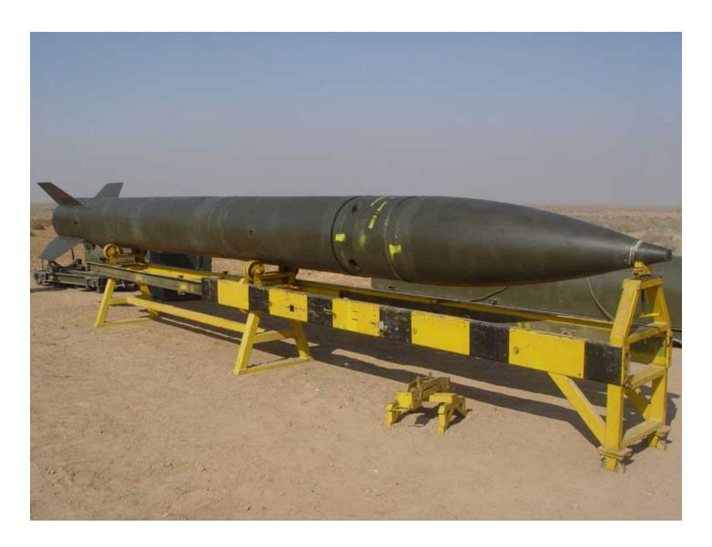
However, the Zelzal was a really long-range artillery rocket with some versions having a range of up to 250km. A CEP of <5% of range in this case would mean about 12.5km which is a truly atrocious level of accuracy.
