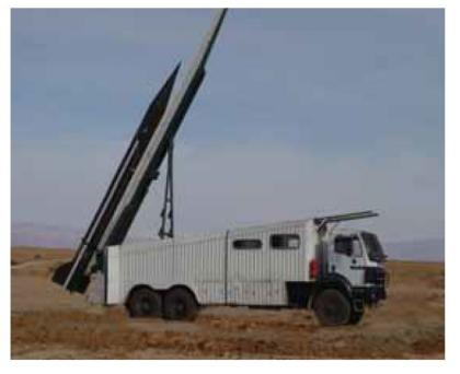
So the Iranians had an idea. Why not stick the guidance system of the Tondar 69 on top of a Zelzal and add some control fins? This would combine the accuracy of the Tondar with the longer range of the Zelzal and its advantage of being both road-mobile and all solid-fuel.
