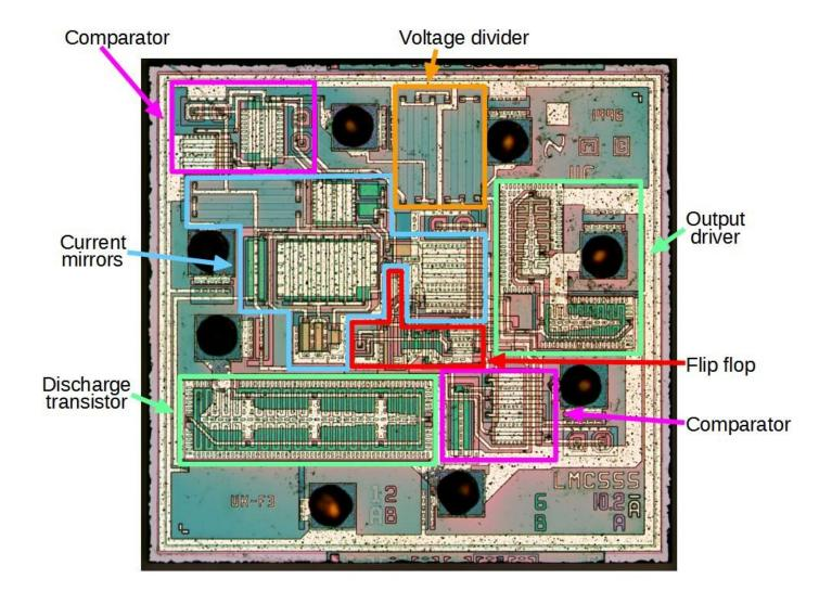
And that's fundamentally a bunch of CMOS transistors (along with some diodes and resistors), which are a type of MOSFET. How many of them are on a 555?
