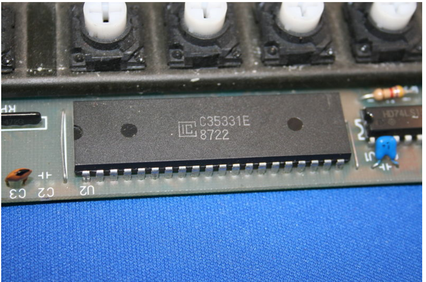
And all keycaps removed! These are "Futaba MA series" (aka Futaba clicky switch) switches.
