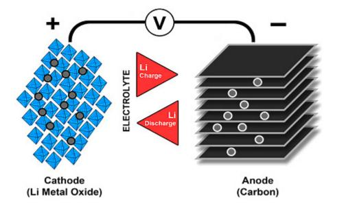
The anode is physically and electronically isolated from the cathode by a separator, often a thin porous plastic film through which the liquid electrolyte permeates.
