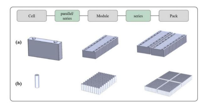
The smallest, but most important, component of the lithium-ion batteries that power EVs is the electrochemical cell,
