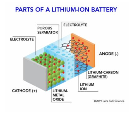
A battery's discharge results from the diffusion of lithium ions from the anode to the cathode through the electrolyte.
