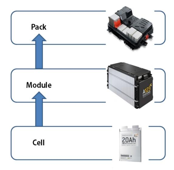
Multiple cells in a case with terminals attached form a module.
