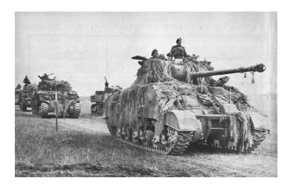
And like the ferocious muzzle blast, even with the muzzle break, could easily obscure observation of the shot's flight - meaning correcting trajectory of APDS rounds was all but impossible.
