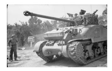
This was really attributed to myriad causes, the much faster/flatter trajectory of SABOT, clipping the muzzle break on firing... and let's not forget the human element, as just firing APDS placed radically different demands on the gunner since the sight was shit. /19
